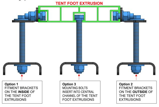
**IMPORTANT**: the supplied nuts and bolts are stainless steel, so it is essential to use an antiseize product on the treads of the bolts (e.g.: Lanotec Type A grease, Nickel Anti-Seize Grease). We also recommend **NOT** to use power tools when tightening the bolts to reduce the risk of seizing an over tightening.
