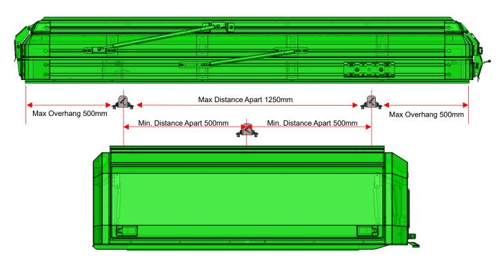
On a ute/pickup, due to the difference in flex between the cab and the tray/canopy, you must not fix the tent across the two, as this will result in damage to the tent and also your vehicle.
